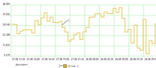
Fig. 9. The graph of the change in the coefficient of unbalance of the current of the negative sequence
